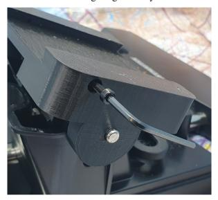
Because you now will be pushing from the front on the pedals and not straight down, its important to look to secure the pedal unit to the floor, or a wooden panel. Use the original supplied fixings brackets. The diagram below is shown on the Thrustmaster Unit.
