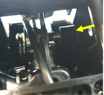
These screws offer no mechanical strength to the set up, they simple act as locking pins to stop the pedals sliding out when not in use. Finger tight is all you need.
