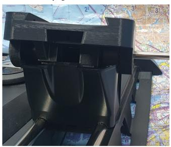
Looking from the other side, gently twist the block so the holes line up and you can see the hinge pin. Push this through so it protrudes evenly on both sides. Turn the unit over and look to see that the mimics lower block is rotating the potentiometer cog. You should see the smooth side of the cog rotating about half a turn.
