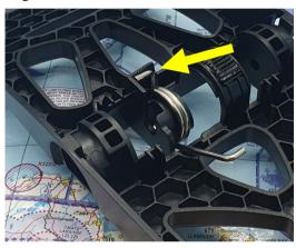
Viewed from the back align the block as shown. Note the location of the spring long leg, which is just hooked inside, and ensure cogged wheel on the potentiometer is pointing upward
