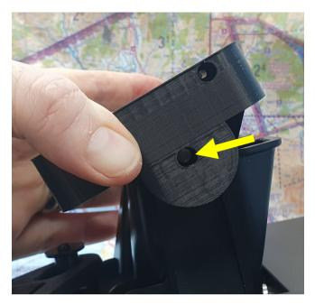
Remove the heel brackets from the original pedals. We will use these screws to secure the new Mimics top pedal.
