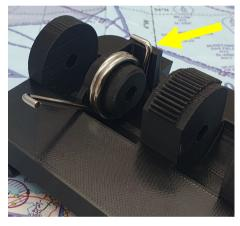
Gentle twist the mimics lower block into the Thrustmaster opening, and use the hinge pin to hold in place. This can be a little awkward, but does not require any strength once everything is lined up. If you are needing to force it, then something is not lined up. Remove and try again
