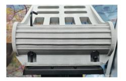
**NOTE**: Ensure the pedal is flush during the tightening. If not loosen the screws before adjusting
