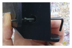
4. Align the screws with the TFRP pedal holes, tighten the first screw (left or right) to about half way then the other side.
