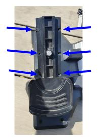
Locate and remove the 6 screws. Three on each side, the blue arrows show the locations.
