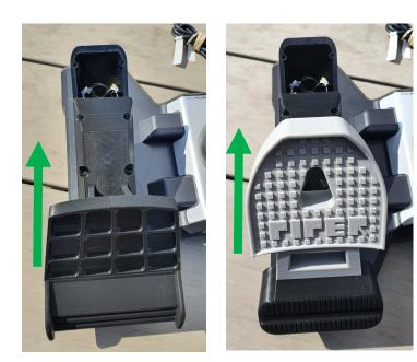
Lay the new pedal on top and slide upwards (Green arrow direction) until hooked. Refit the top four screws. ensuring the cables are free and not trapped.
