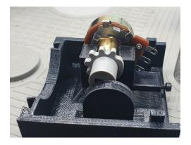
Secure the potentiometer into the main body side wall. You will need to straighten the contacts to prevent fouling of the case. Note the key way for the lug, and the potentiometer will click into place.
