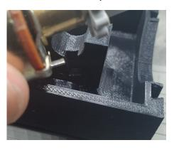
Twist the small grey cog so it aligns as shown the picture above. When the wall shell is slid onto the main body the cog will need aligning. Holding the two pieces together test the rotation, you can plug in the unit at this stage and test the braking output.
