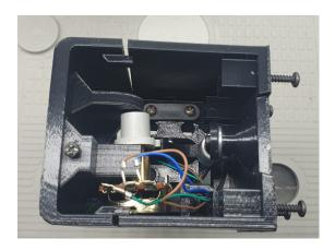
Ensure all cabling is free from snags. Fit the remaining 15mm screw to tap out the hole, remove and fit the lid by locating the tapered edges.
