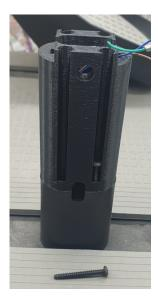
Using four of the 25mm screws, secure the post extender routing the cables through the middle.
